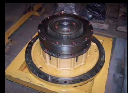
D11R Steering Clutch & Brake unit. Fully rebuilt Part No 1299234. $14,000 + GST stand incl
