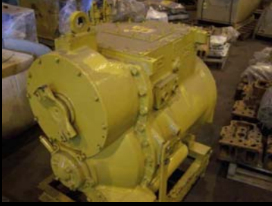
769C Transmission. Rebuilt and tested by Cat Dealer Suits 1X1-UP. Part No 7G1140 $46,000 + GST
