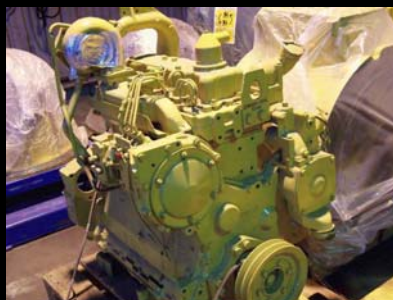
3304 DI Engine. Suits 120G. Fully rebuilt Serial # 11W, 72V-UP. Part No 7N1131. $ 16,000 + GST
